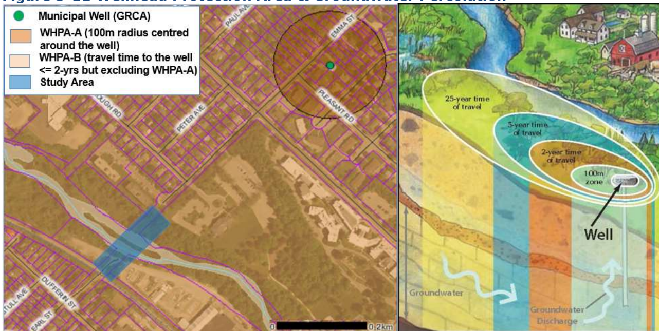
Figure 3-11 Wellhead Protection Area & Groundwater Percolation
